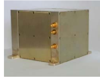
Fig. 1: The USO, an Ultra-Stable-Oscillator, 15x13x10cm 3 , based on quartz resonator
