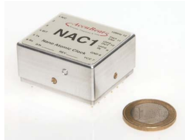
Fig. 1: Photograph of NAC1 with the dimensions of 41 \times 35 \times 22 \text{mm}^3 , power consumption of 1.2W, demonstrating a frequency stability (ADEV) of 8 \cdot 10^{-12} at 1000s, and an aging of 3 \cdot 10^{-10} per month.
